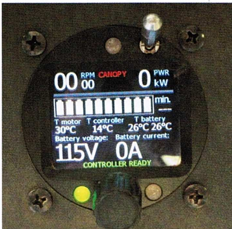
The motor is controlled by a FES Control Unit instrument (FCU), located in the instrument panel. It was designed to simplify FES operation.
