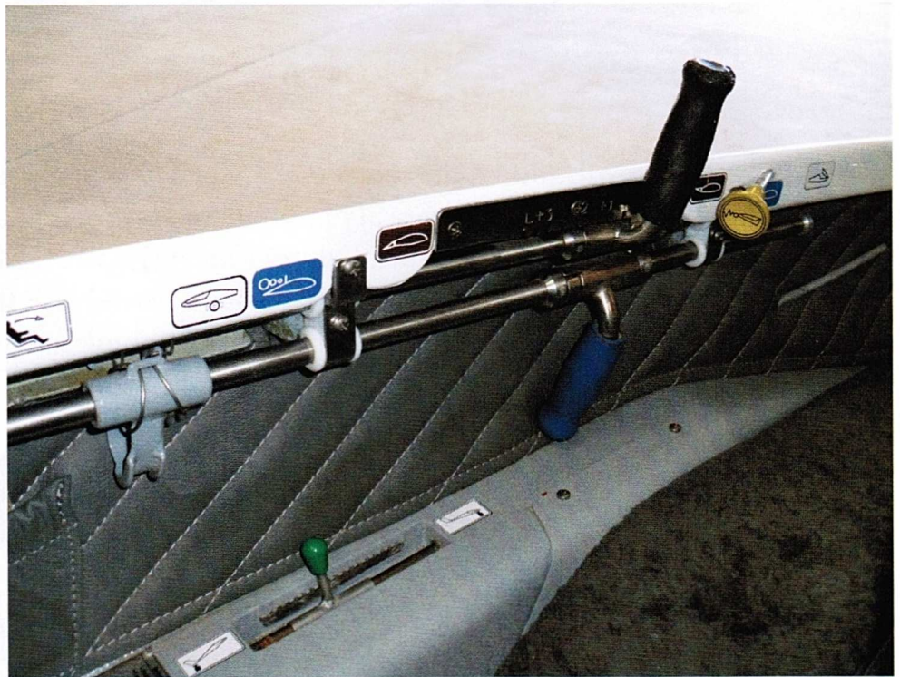
Fairly standard placement of controls for flaps, trim, water management and rudder pedal adjustments are found along the cockpit sides. Red safety cover is for the Power Switch.
