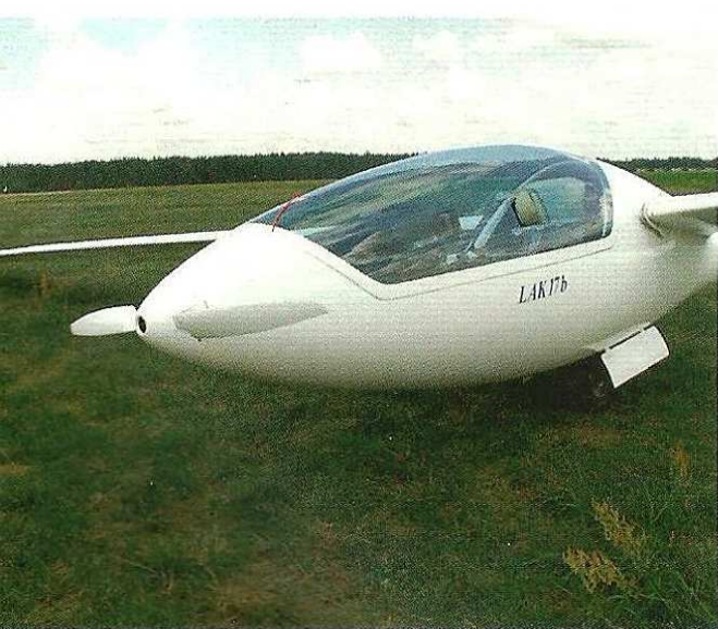
(Above and below) The Front Electric Sustainer system: an electric motor with foldable propeller can be started at a low altitude (photos courtesy of Baltic Sailplanes)
