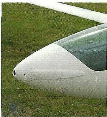
(Above and below) The Front Electric Sustainer system: an electric motor with foldable propeller can be started at a low altitude (photos courtesy of Baltic Sailplanes)
