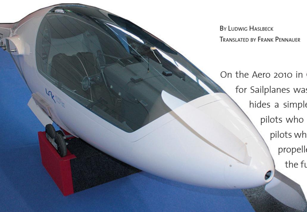
On the Aero 2010 in Germany a new propulsion concept for Sailplanes was introduced. Behind the name FES hides a simple idea which is known to all glider pilots who were at one time also model plane pilots where an electric motor drives a folding propeller which is mounted on the nose of the fuselage.
