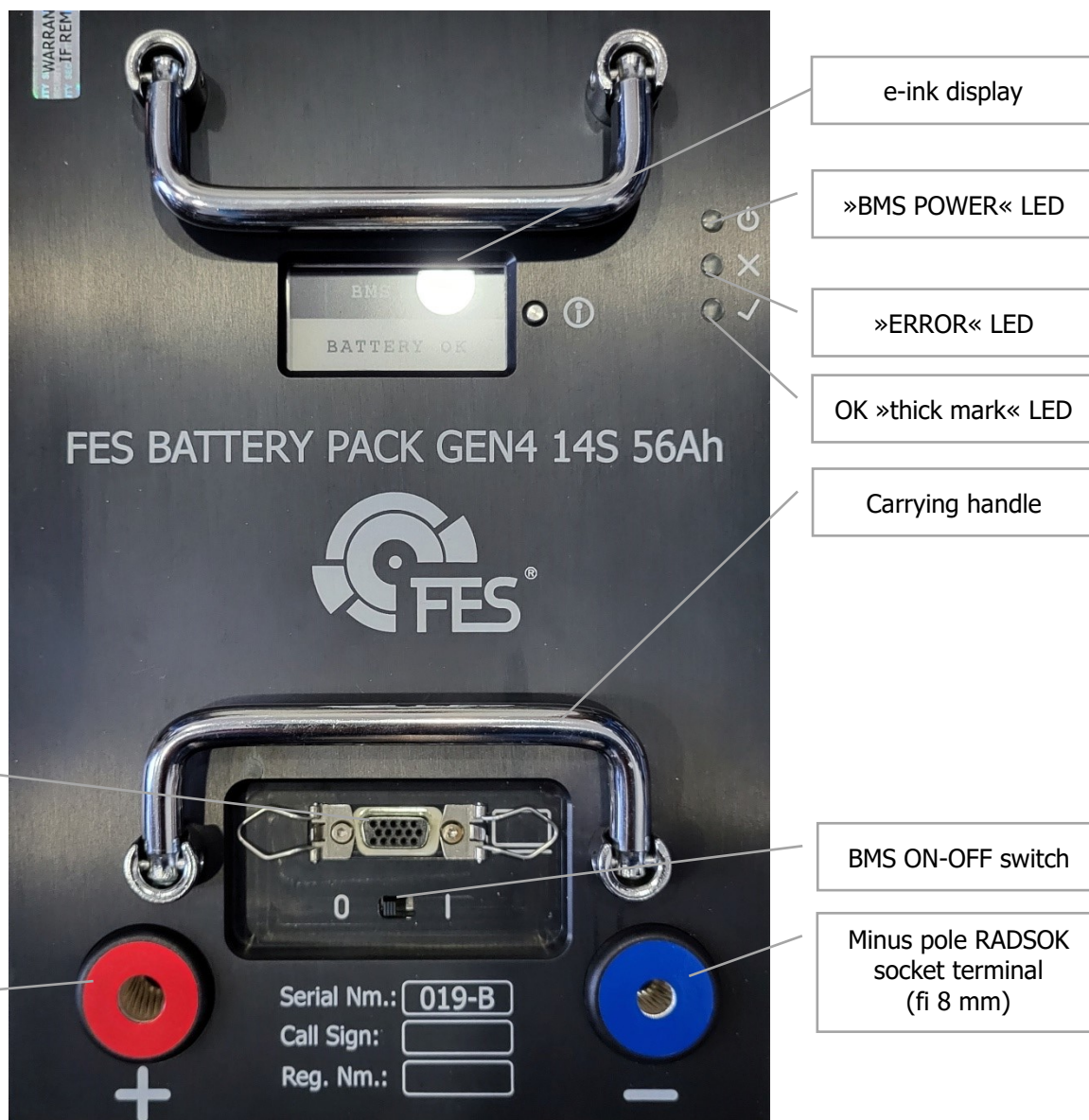
Top view of FES GEN4 14S 56Ah Battery pack
