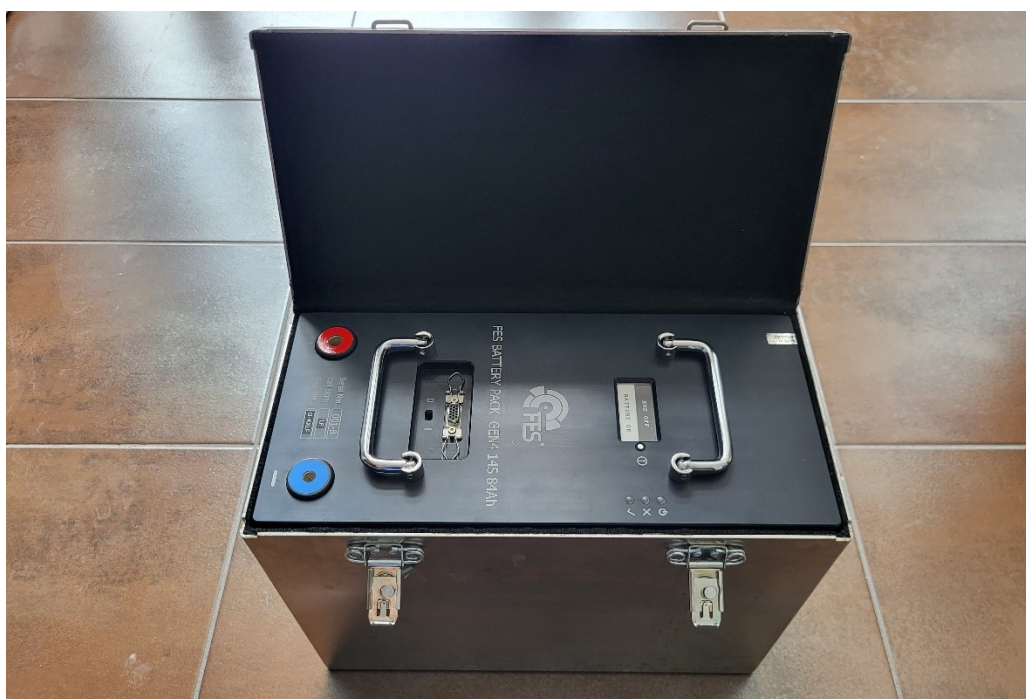
FES GEN4 Battery pack placed into FES Stainless steel box
