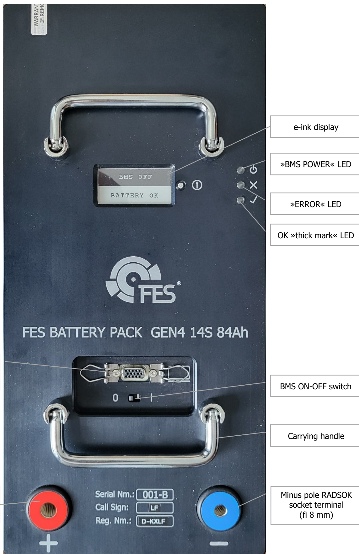
Top view of FES GEN4 14S 84Ah Battery pack
