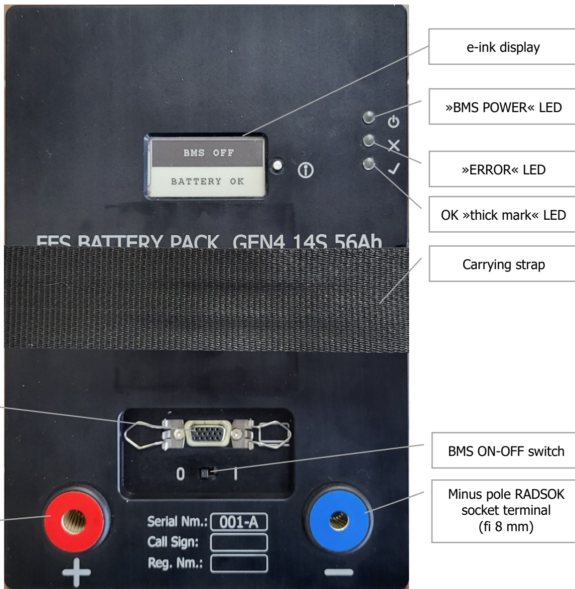
Top view of FES GEN4 14S 56Ah Battery pack
