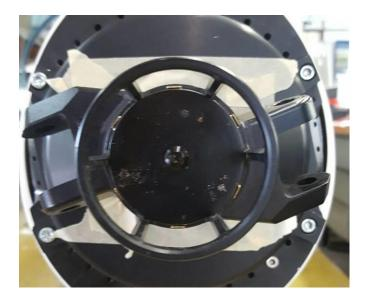
2. Before starting removal process of propeller blades it is strongly recommended to close motor openings with a tape, as show on photo above to prevent any of the small parts entering the motor, if it falls through the fingers by coincidence. When this happens, it is usually necessary to remove and open motor, which is quite demanding job, so it is much easier to tape openings.
