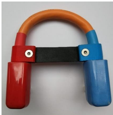
Top and bottom view of right-angle type of "Connecting cable", as used on LAK gliders.
