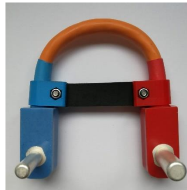
Top and bottom view of right-angle type of "Connecting cable", as used on LAK gliders.
