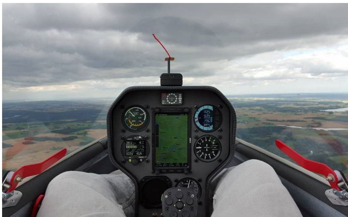
Suitable position for FCU instrument on the panel of Silent 2 Electro
