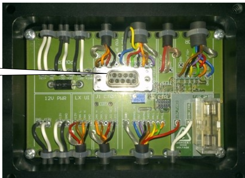
FCC (FES connecting circuit) with cover removed
