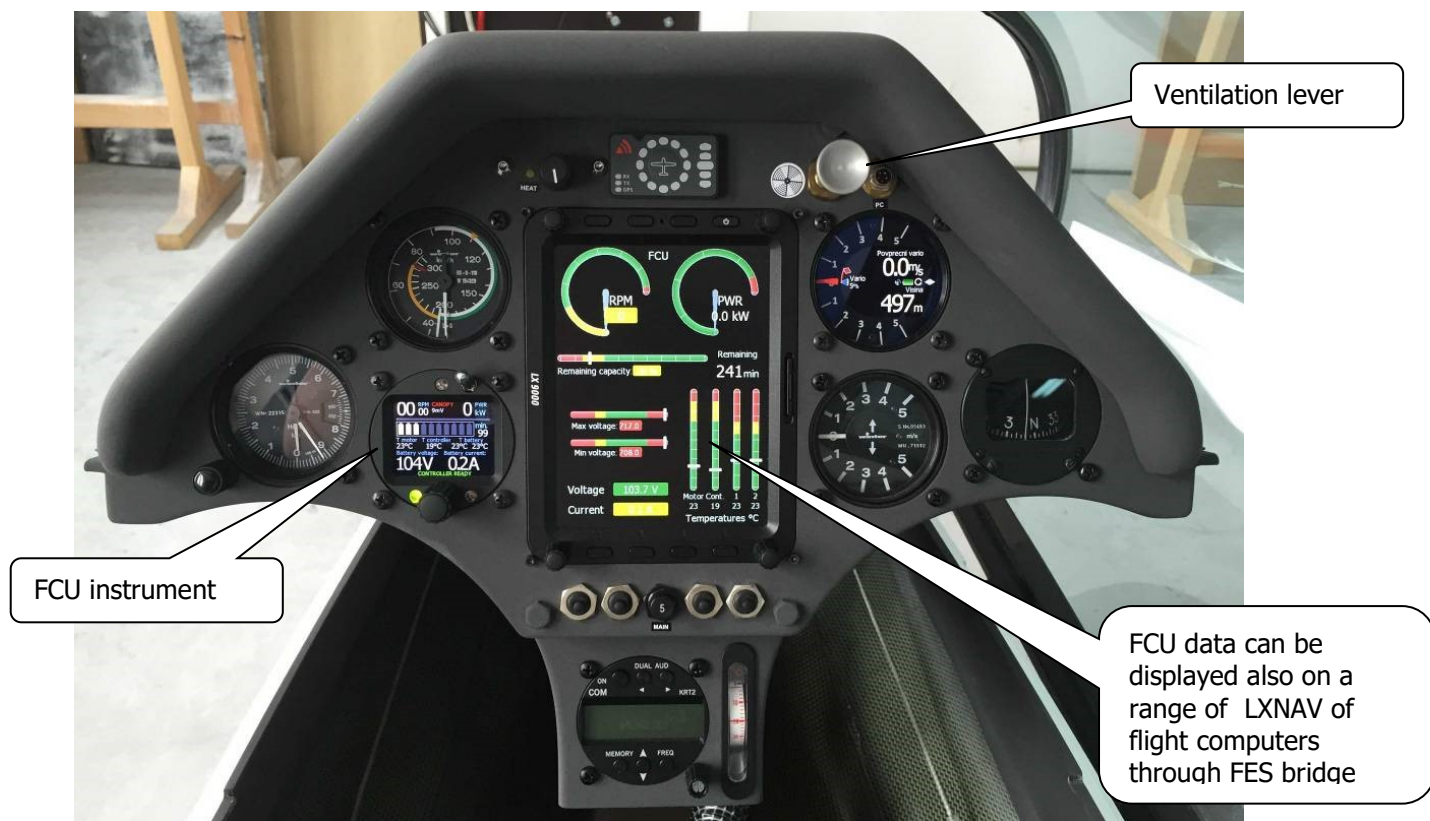
Suitable position for the FCU instrument on the panel of Ventus 2cxa FES
