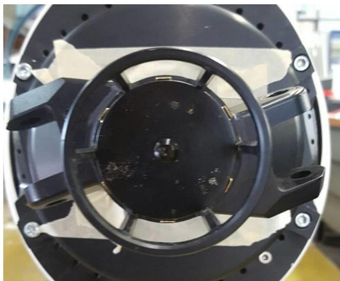
4. Before placing washers, crown nuts, and split pins, it is strongly recommended to close motor openings with a tape, as show on photo above in order to reduce possibility that any of the small parts could enter the motor, if it falls through the fingers by coincidence. If this would happen, it is usually necessary to remove and open motor, which is quite demanding job, so it is better to tape openings.
