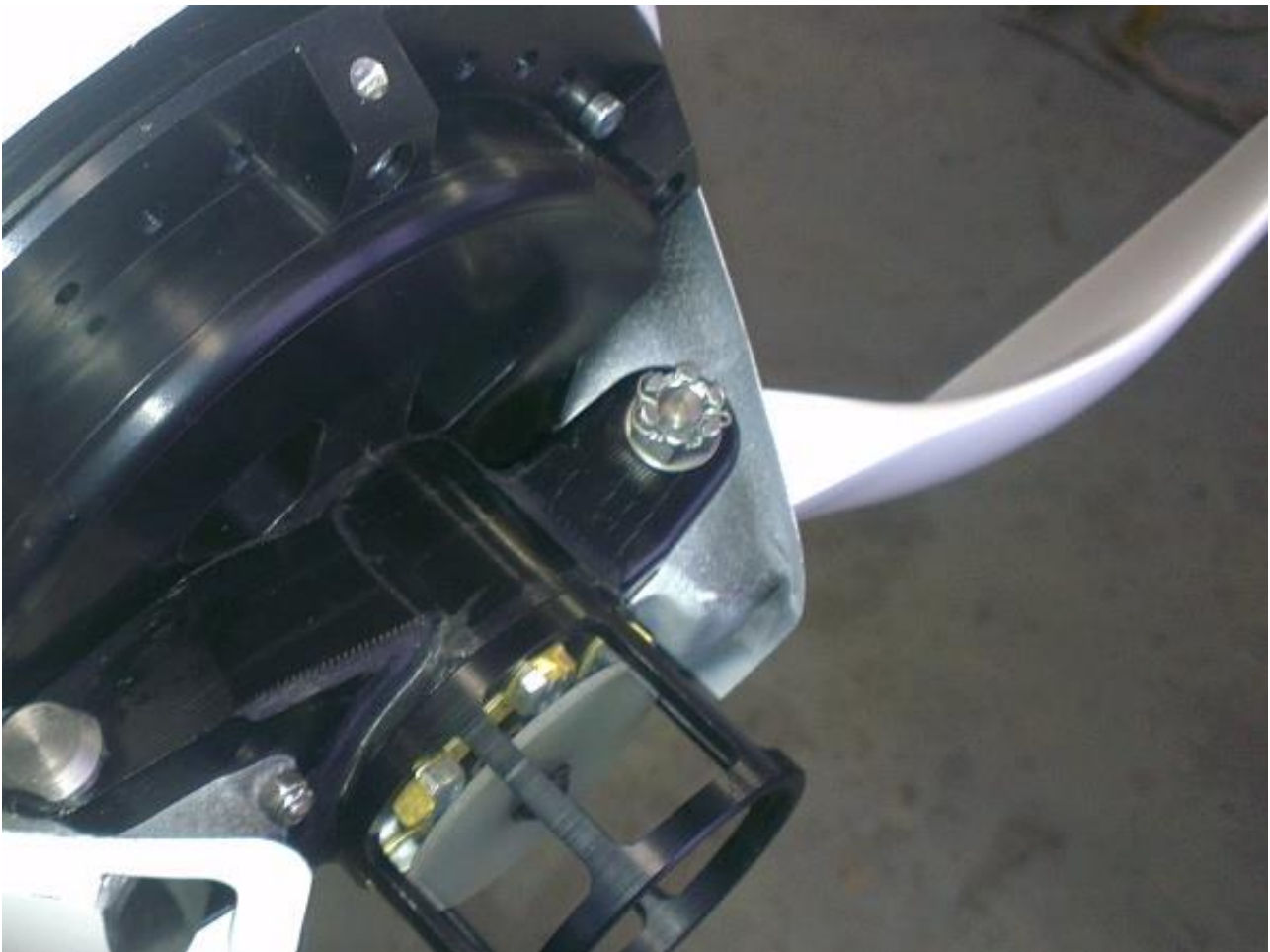
Fig.1 Propeller blades mounting on the holder
