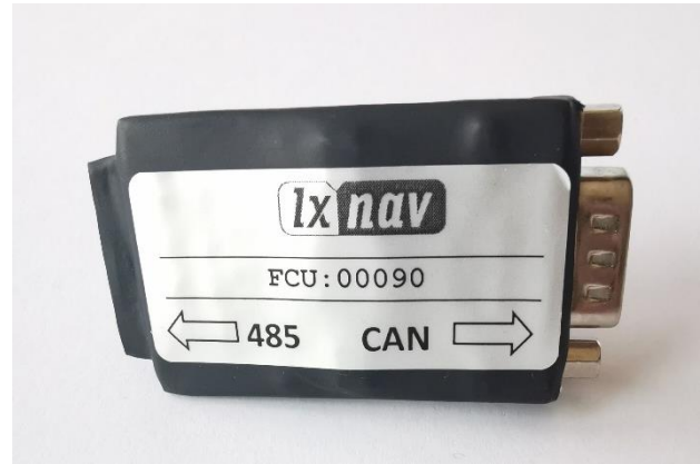
FES Bridge, back view
