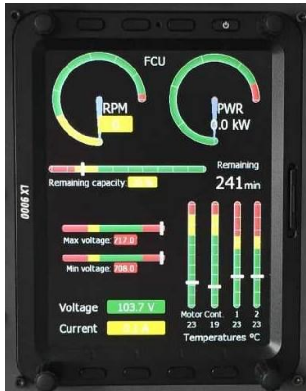
FES system data on LX9000 with "Power switch" ON
