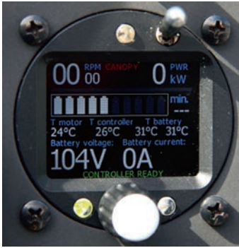
FES control unit
