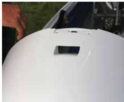
Air extractor: Ventilationen bakom cockpit.
