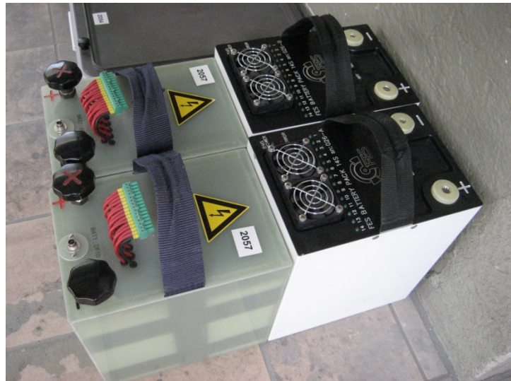
Two batteries of the previous design (on the left) and two batteries of the latest version with integrated charge controllers (on the right).
