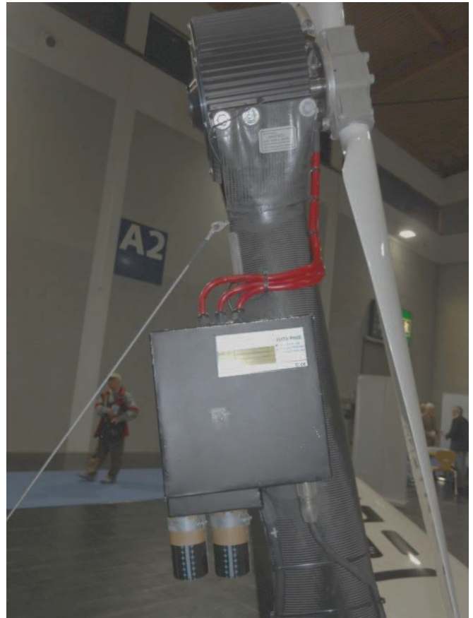
Early-type 40KW electric power plant
