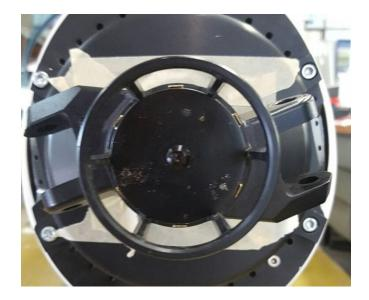
2. Before start of propeller blades removal it is strongly recommended to close motor openings with a tape, as show on photo above to prevent that any of the small parts could entering the motor, if it falls through the fingers by coincidence. When this happens, it is usually necessary to remove and open motor, which is quite demanding job, so it is much easier to tape openings.
