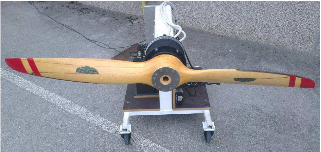
Motor mounted on test bench with a wooden propeller
