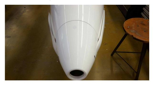
7. Fix the spinner with four Inox M4x8mm countersink head screws, and two M4x6mm screws. **Two screws which are 2mm shorter are located at 60deg and at 300deg angle (upper left and right).** Tightening of all 6 screws should be gently with small torque (do not use high torque, as thread in the aluminum plate could be damaged). Please do not use any glue to secure them, as during rotation centrifugal force to the
