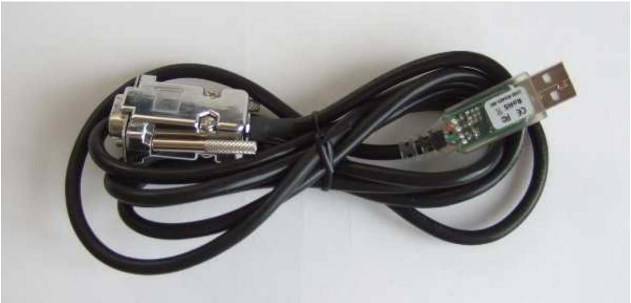
BMS-PC communication cable (suitable for external BMS, GEN1 battery packs)
