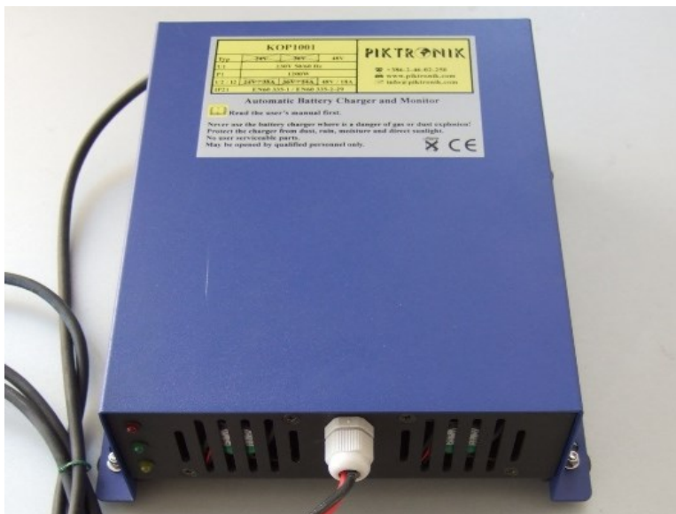
KOP1001 BMS Charger
