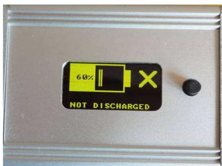
By pressing button, it will start discharging of battery pack through electric radiator. A text "DISCHARGING" and an arrow symbol will be displayed.
