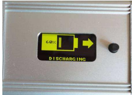
When battery pack voltage will reach 50% of charge (51.8V, 3.7V/cell) a device will automatically disconnect electric radiator from the battery pack, which will prevent further discharging of the battery pack.
